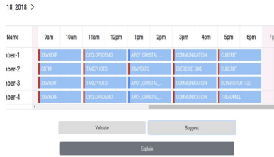
Figure 3: Suggesting the user a completion for their partial input schedule. Tasks added by CAP have a left red border.
